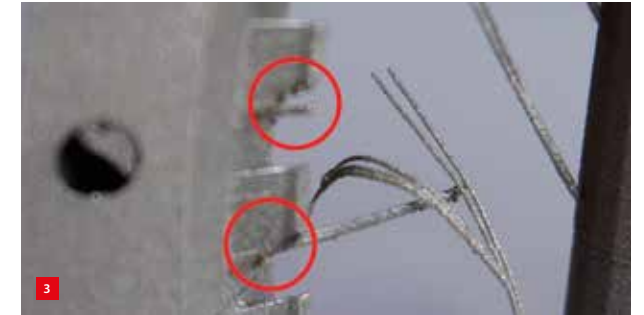
2) Fragile branches in the tree structure which have unfortunately snapped (see Figure 3).
