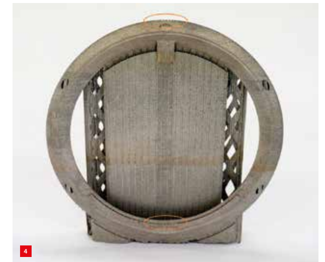
4 Result of the second print job, with optimised support structures and adjusted seal design.
