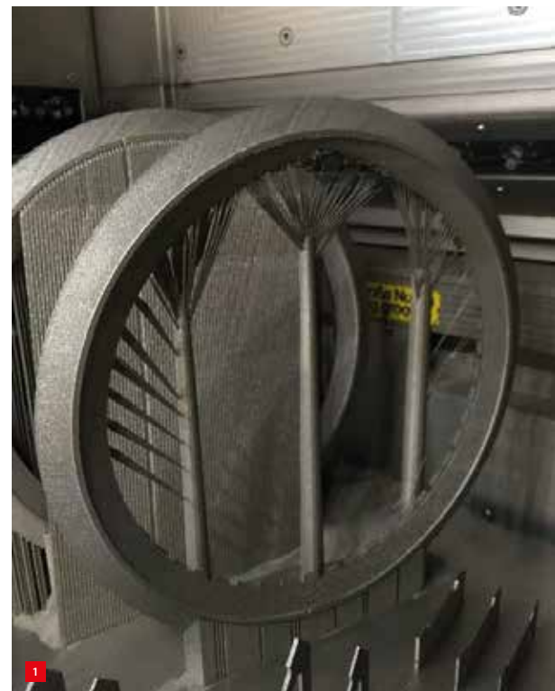
1 Single seal printed in an upright position supported by the so-called tree structures. In the back, the same seal can be seen printed with full supports. For this last type of support, note the undesirable amount of printing powder that remains after cleaning.
